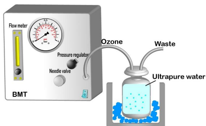
Figure: Scheme of the ozonization
