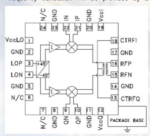
Corporation (model HMC597LP4E). A modification in the bias network has to be implemented to allow In-Phase (I) and Quadrature-Phase (Q) output down to dc. The I/Q-output signals have to be amplified by high speed differential amplifiers with dc level shift (AD8132). The complete circuit provides various features which have to be tested and investigated with respect to the critical requirements of an amplifier control loop.
