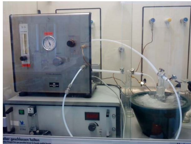
Generator for ozone stock solution
