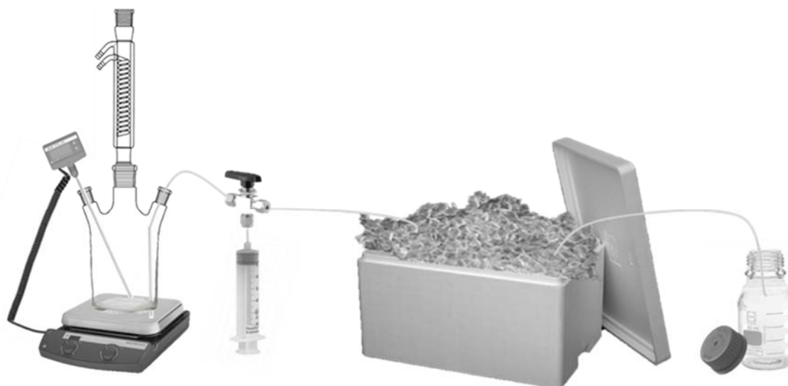
Figure 1 Experimental set-up to investigate the mineralization products of nitrogen containing compounds by sulfate-radicals.
