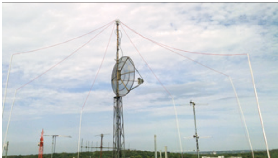
Figure 1 — Inverted V wire switched beam array antenna on the roof platform. The dipole wires have been colored for better visibility.
